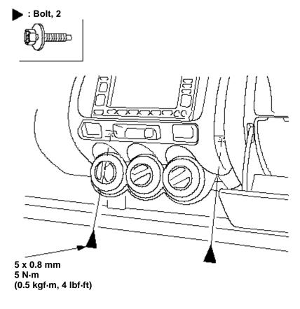
6. Using a wrench, carefully insert a wrench from the inner glove box opening, and push a panel clip on the glove box side from back of the center panel (A) to release it. LHD is shown, RHD is symmetrical.
