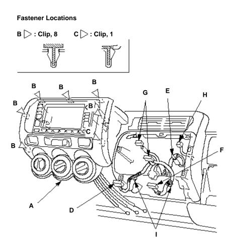
8. Install the panel in the reverse order of removal, and make sure each connector is plugged in properly, and antenna lead and cables are connected properly.
