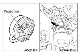
Align the projection on the oil pump case (arrowed part) that prevents the turning of the engine oil cooler with the projection on the engine oil cooler, and install the engine oil cooler.
