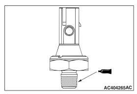
1. Apply the specified sealant to the thread of oil pressure switch.
