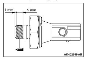
7. Apply the specified sealant to the thread of oil pressure switch.
