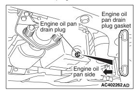
4. Install a new drain plug gasket so that it faces in the direction shown in the illustration, and then tighten the drain plug to the specified torque.
